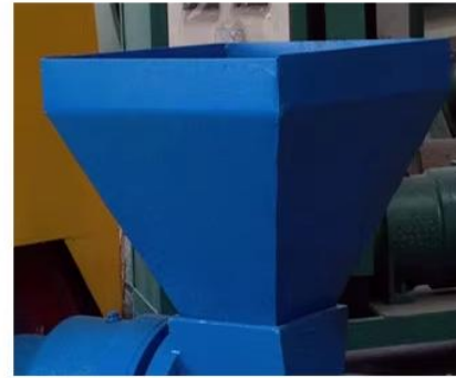
Lengthened, widened and deepened steel inlet
